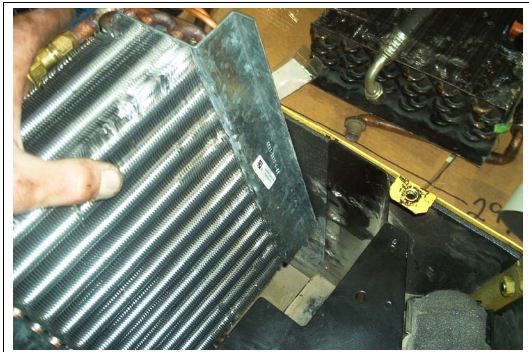
Screw the A/C coil to the heater assembly flanges so the top of the coil is just below the top of the flanges. Use the self drilling screws provided. Screw the coil to the flanges outside the box and then re-assemble after the bulkhead lines are installed.
