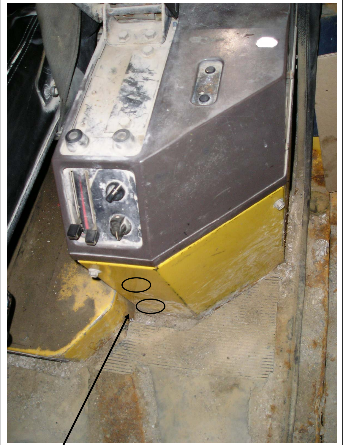
Add ball louvers to this panel for increased air flow in the cab.
